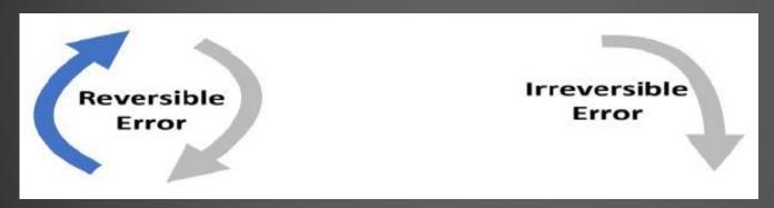
A well-designed system or procedure should mean that errors made by aircraft maintenance technicians are reversible. Thus, if a technician installs a part incorrectly, it should be easily spotted and corrected before the aircraft is released to service by the supervisory procedures in place.
