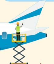
Engage parking mechanism, parking brake or install wheel shock when GSE is stationary position.
